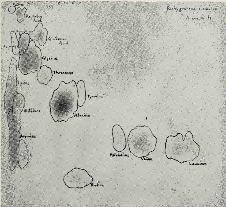
FIG. 4. Chromatogram of free amino acids of Pachygrapsus crassipes from Anacapa Island, a nonpolluted area.
